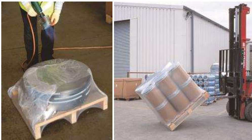
Figure 5 – Appliance of the Polyethylene Shrink and Durability of the Pallet with Polyethylene Shrink
