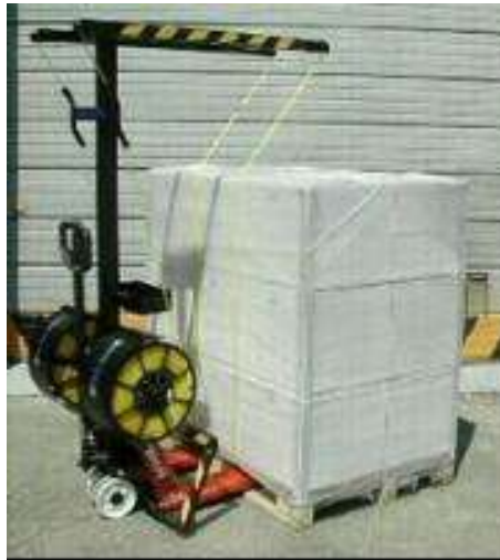
Figure 7 – Application of the Pallet Strapping
