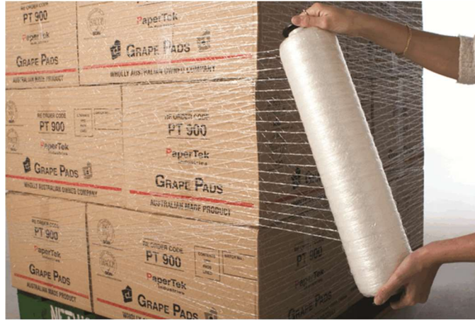
Figure 6 – Wrapping Film (Stretch Film) Technique
