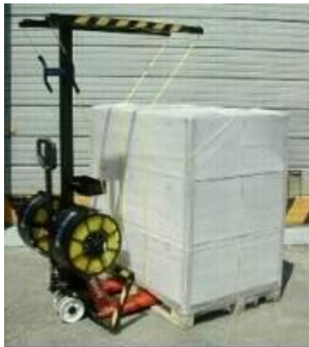
Figure 7 – Application of the Pallet Strapping
